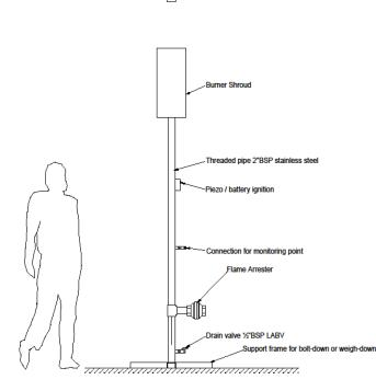
Landfill Systems manufacture both manual and automatic ignition versions of their successful range of Environmental Gas Flares.
